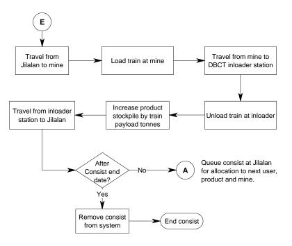
Figure A2. Flowchart for sending a train to a mine
